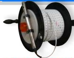
Contact Meter Typ KLL 15-50m with hand-drum
